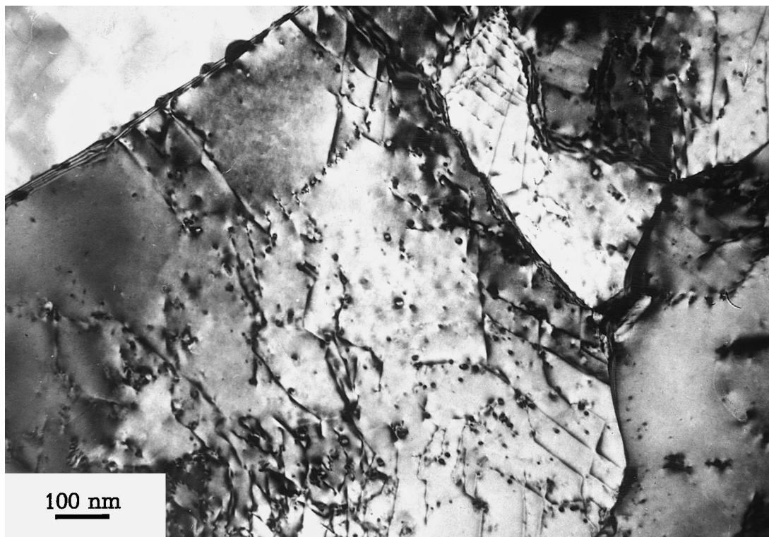
Fig. 6. Radiation defects in irradiated RPVS: “black dots” and dislocation loops (bright field image, F = 6.5 \cdot 10^{23} n/m 2 ),
